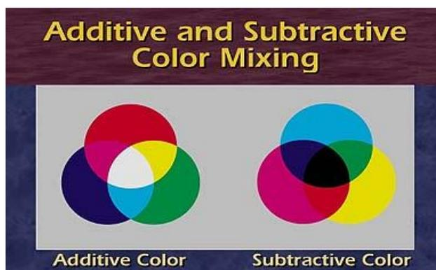
The offset printing process uses **Cyan**, **Magenta** and **Yellow** (which are the secondary additive colours) process colour inks and a fourth ink, **Black**, designated 'K' to avoid confusion with 'B' for Blue or Black. By overprinting one transparent printing ink with another the secondary subtractive colours produce **Red**, **Green** and **Blue** which are the additive primaries.
